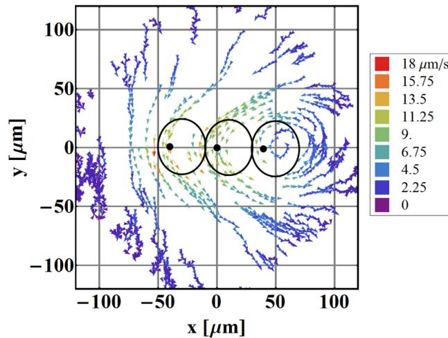
FIG. 6. Mapping of fluid flow around three linearly arranged artificial cilia. Black dots denote the anchoring sites and the solid lines the calculated paths of the tips of the cilia.  $\omega/2\pi = 2$  Hz;  $L = 30.8$   $\mu\text{m}$ ,  $\psi = 49.6^\circ$ ,  $\vartheta = 30.4^\circ$ ,  $z = 40$   $\mu\text{m}$ . The velocity scale is different than in other images due to larger pumping effects.
